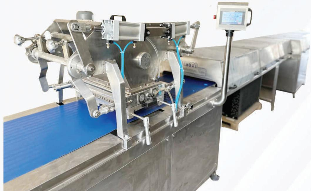
A machine for pouring chocolate (drops) in different sizes and weights, with a large production capacity. Equipped with a cooling tunnel available with two operating systems (servo motors, air silencers), with PLC control screen. Drupes are used in baked goods, cake molds, and decorations.
